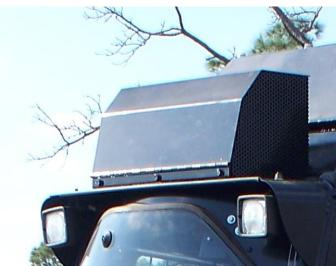
Supertrak is proud to offer an Industry First Air Pressurizer Kit for your Caterpillar® C-Series Models. The Air Pressurizer Kits reduces the amount of dust and debris that enters the cab by introducing filtered fresh air while operating in severe dusty environments such as applications like Forestry, Grading, or Recycling.
